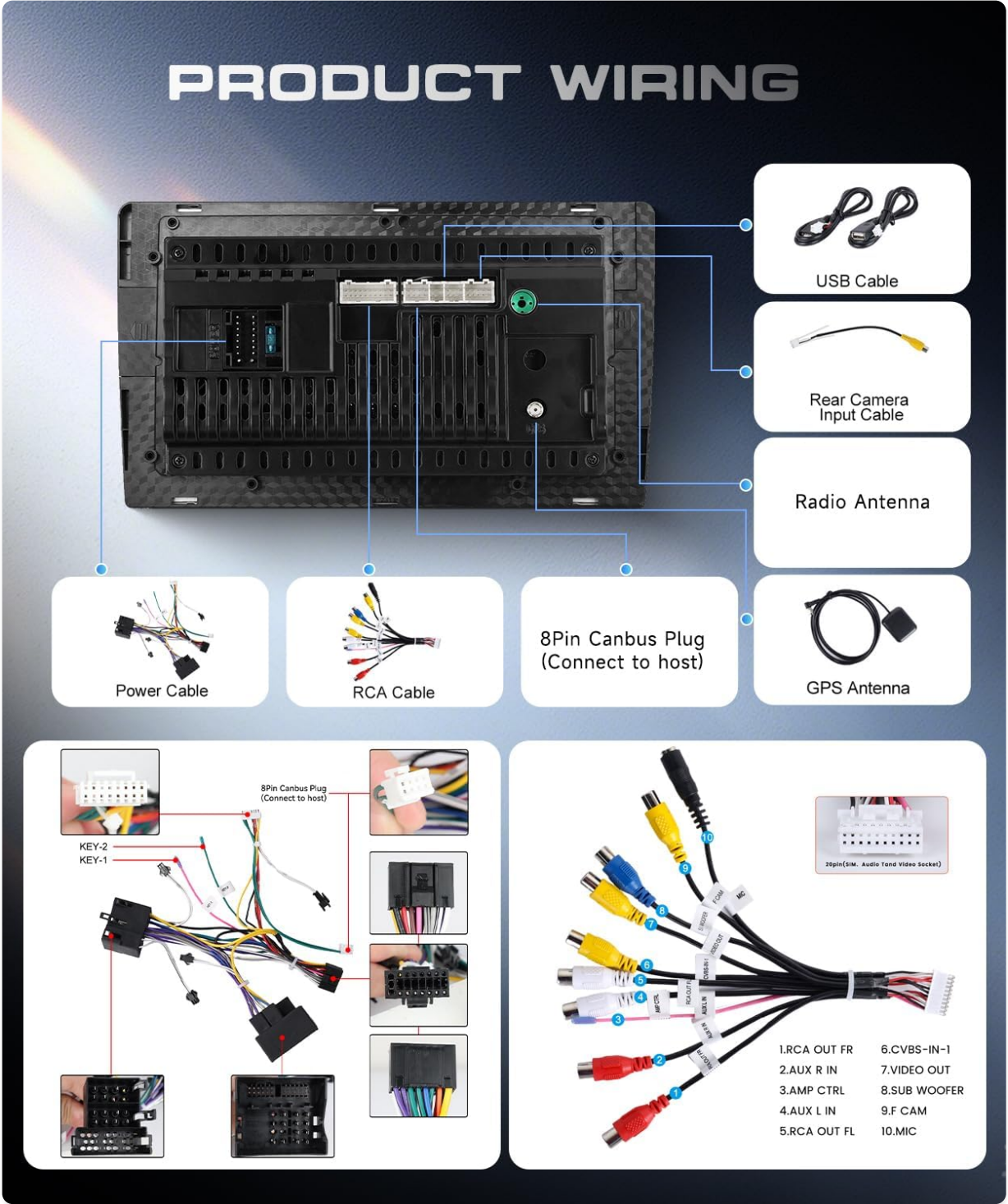
Image: Detailed diagram illustrating the connections for power, RCA, USB, radio antenna, GPS antenna, rear camera input, and CAN-BUS.
