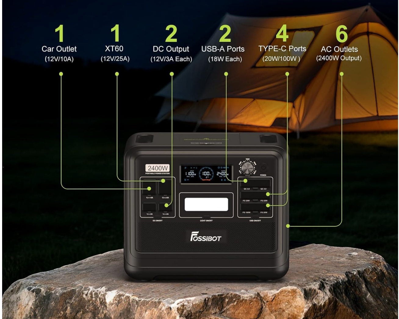
Image 4.1: Overview of the F2400's 16 output ports, detailing their types and locations.
