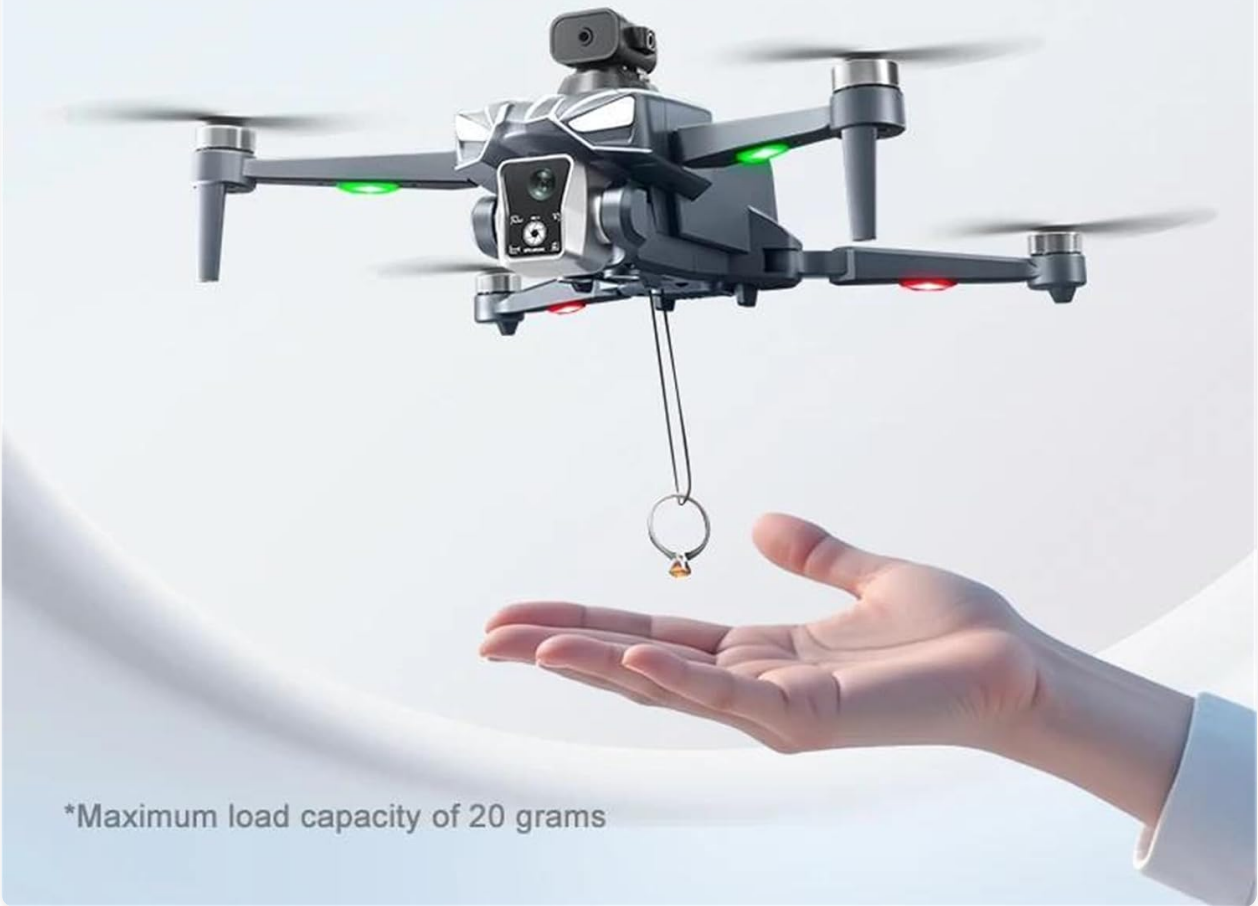
Image 5.3: The drone demonstrating its one-click airdrop capability, releasing a small ring from its payload mechanism.
