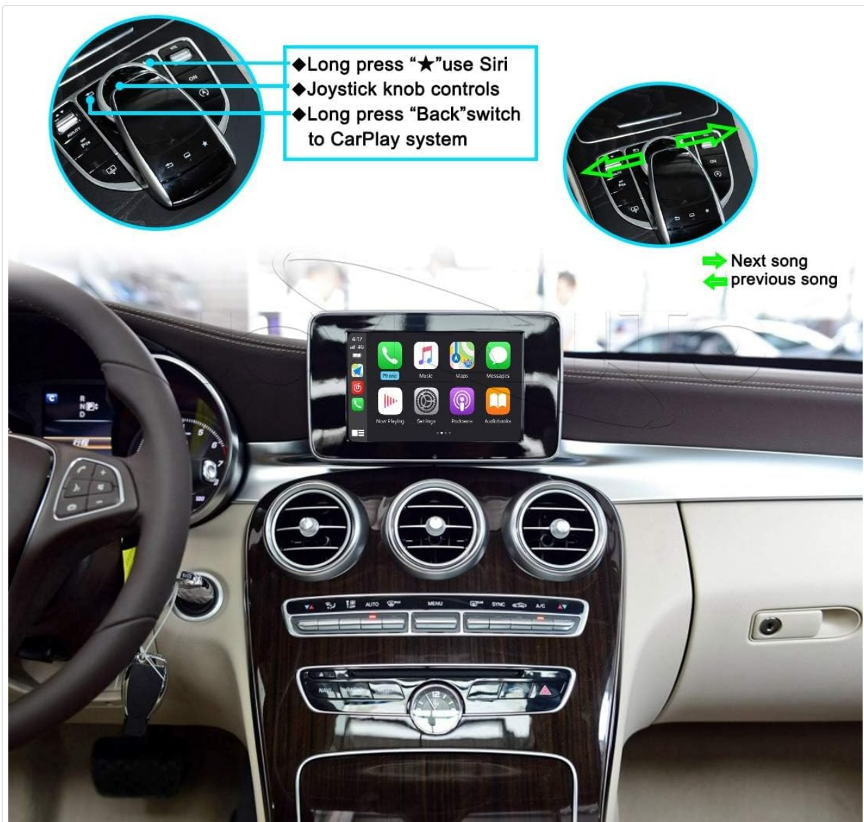
Image: An illustration highlighting how to use the original steering wheel buttons and joystick knob to control the CarPlay system, including activating Siri and switching between systems.
