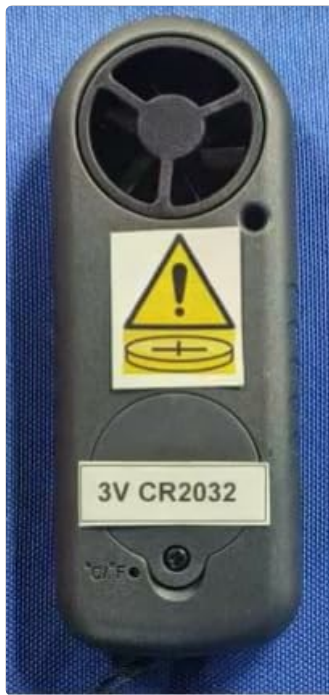
Figure 5: Location of the °C/°F temperature unit switch.
