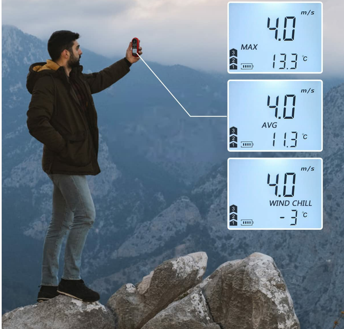
Figure 4: The anemometer displaying different measurement modes: MAX, AVG, and WIND CHILL.
