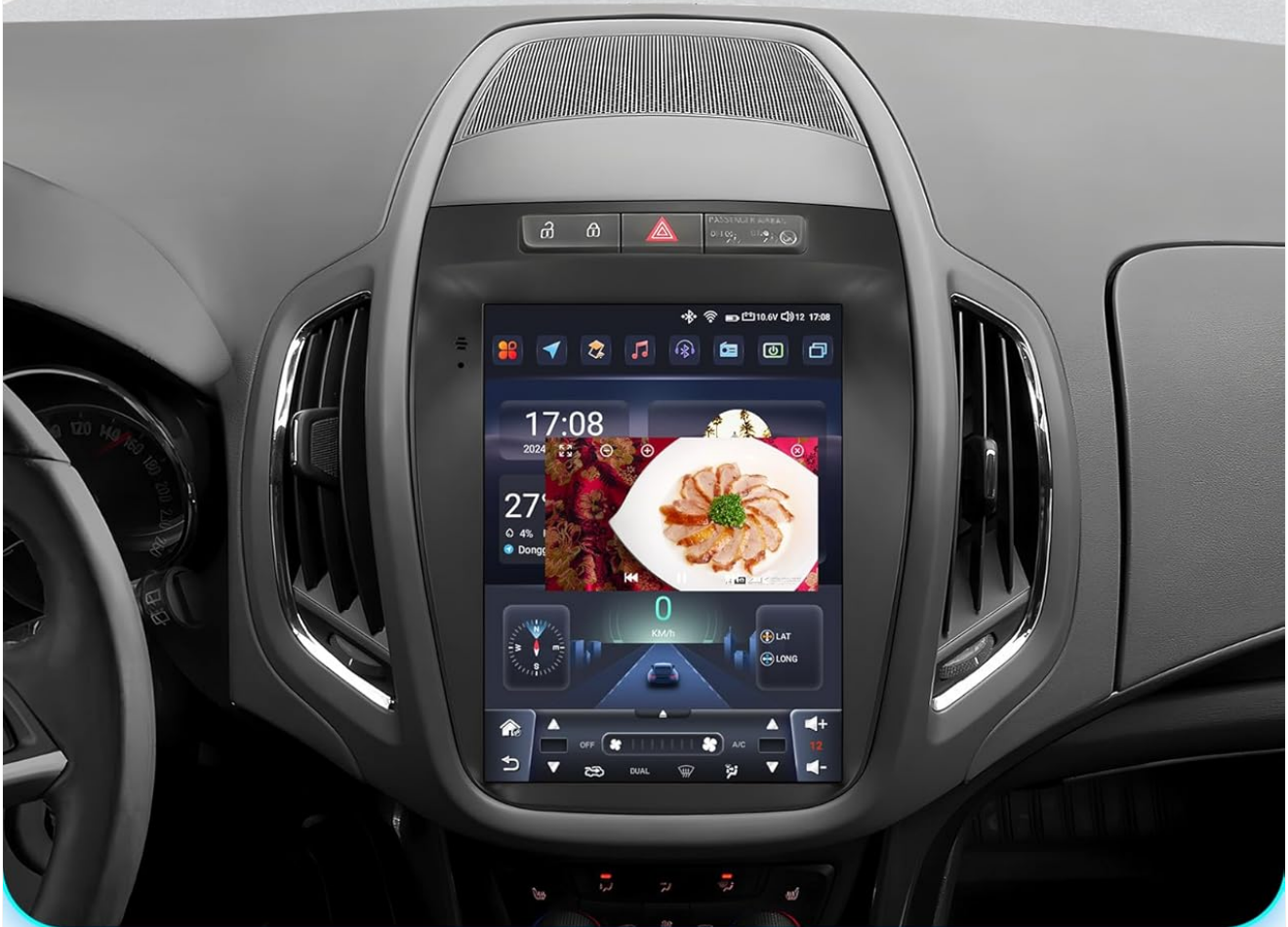
Image 4.5: The car radio display demonstrating the Picture-in-Picture (PIP) feature, where a video plays in a small, adjustable window while other applications are visible.
