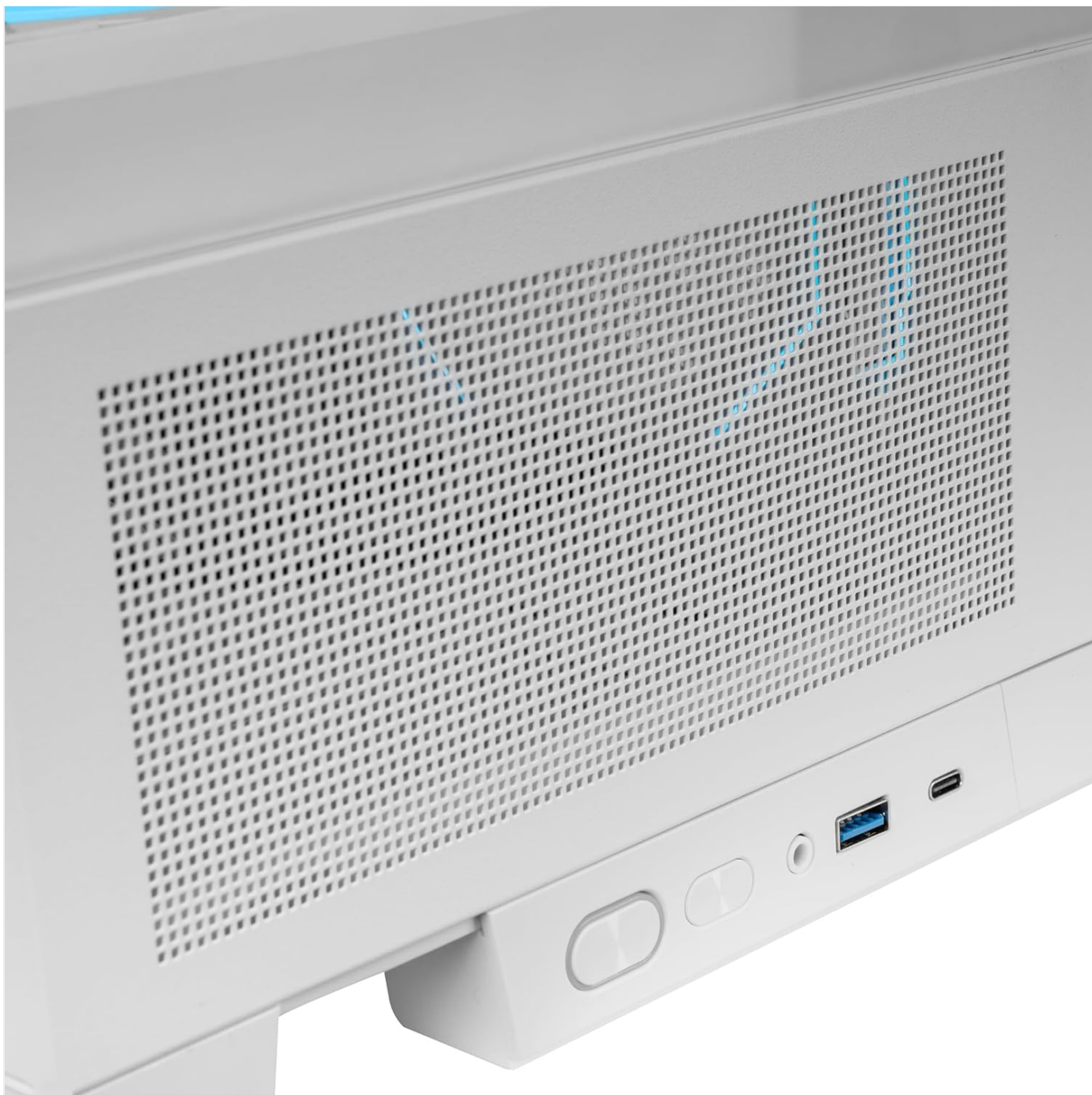
Image 7: A close-up of the Mars Gaming MC-LCDX's front I/O panel, showing the power button, USB ports (including USB-C), and audio jacks for convenient peripheral connectivity.
