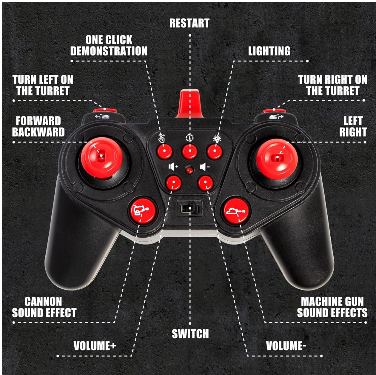
Image 2.1: Remote Controller Layout and Functions.
