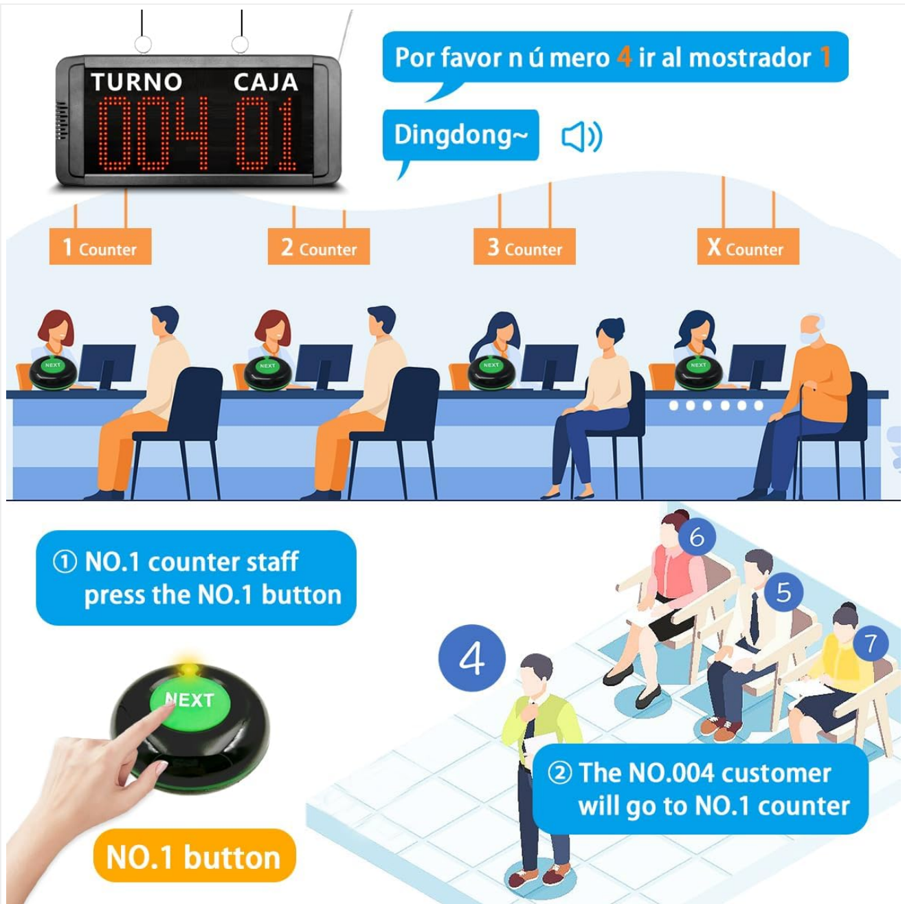
Figure 1.1: System Operation Overview. This image illustrates how the queue system functions, from a staff member pressing the 'NEXT' button to the display showing the current number and the customer proceeding to the counter.
