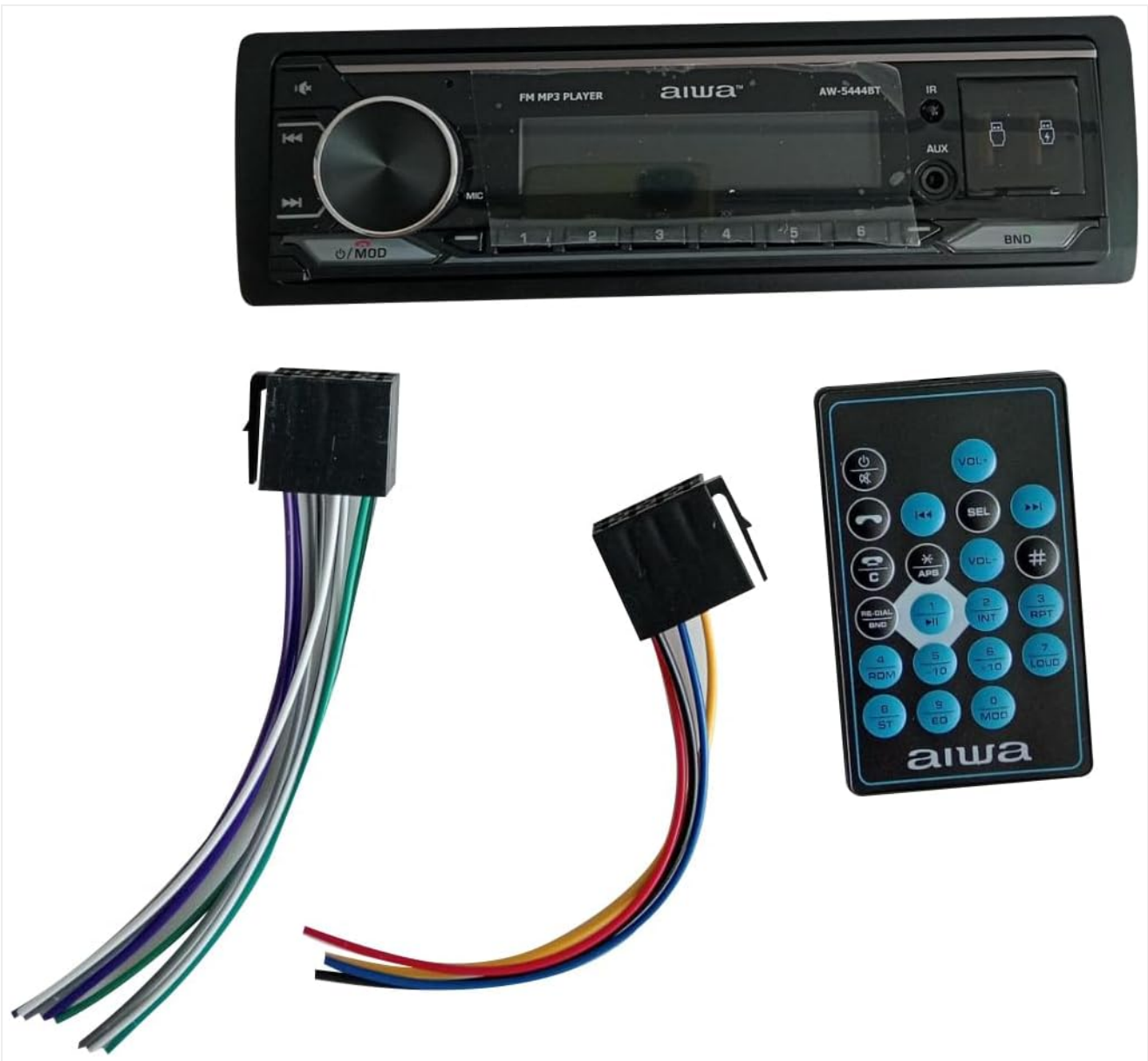
Figure 3.1: Included components of the Aiwa AW-5444BT car stereo system.
