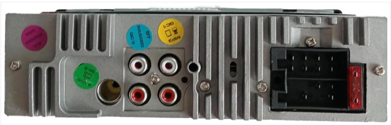
Figure 4.2: Rear connections of the Aiwa AW-5444BT Car Stereo.
