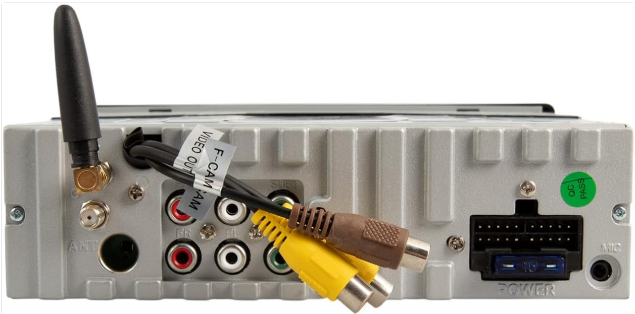
Figure 2: Rear Connections. Illustrates the various ports for power, speakers, camera, and auxiliary devices.
