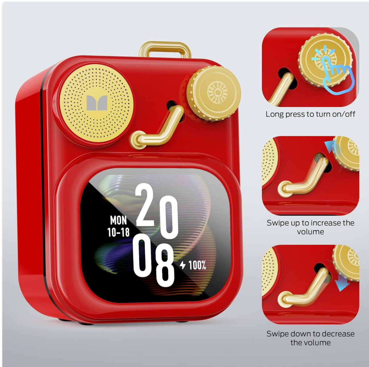
Image 3.1: Power On/Off and Volume Control via the top right knob.
