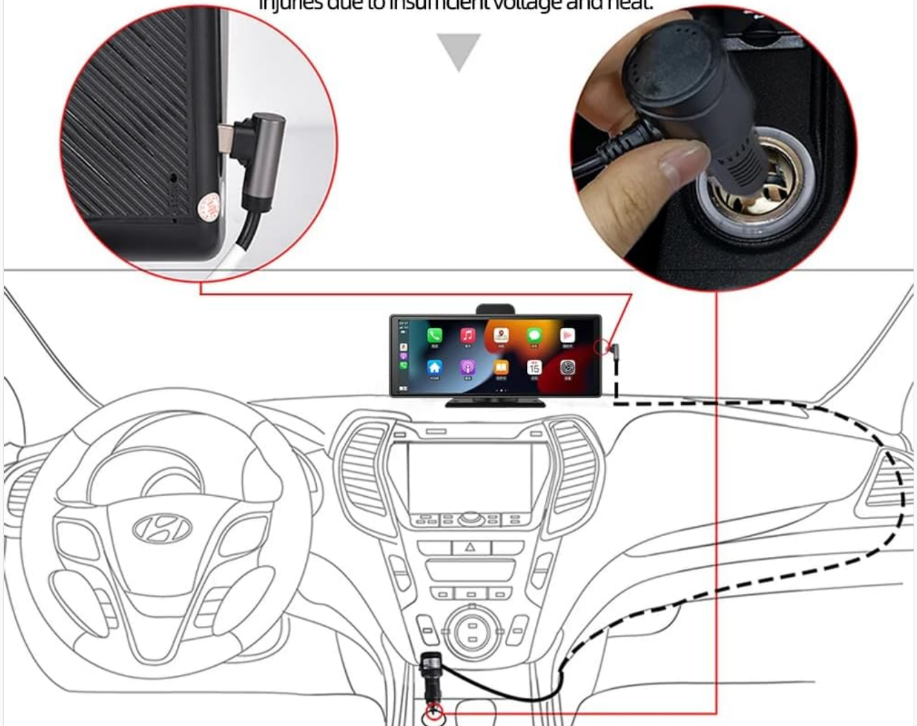
Image: Wiring instructions for connecting the car stereo to the vehicle's power source.
