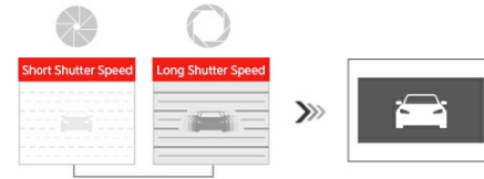
Figure 3.2: Dual HDR processing ensures balanced exposure in challenging lighting conditions.
