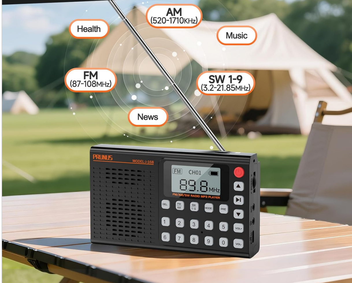
Figure 3.1: Front view of the PRUNUS J168 radio, showing the digital display, keypad, and control buttons for various functions.
