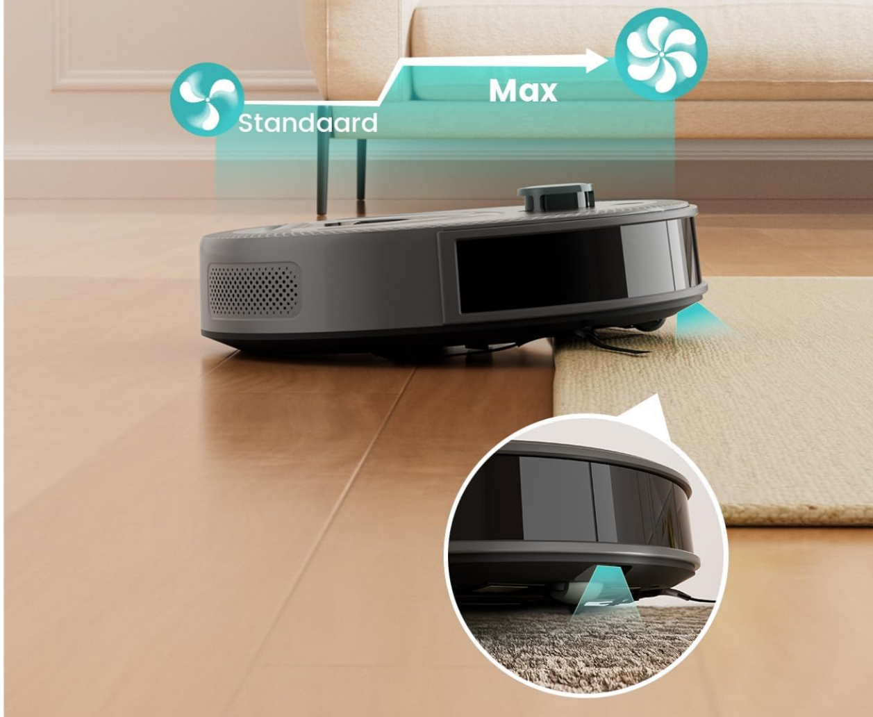
Image: The LEFANT M330Pro demonstrating automatic suction power increase when transitioning from hard floor to carpet.
