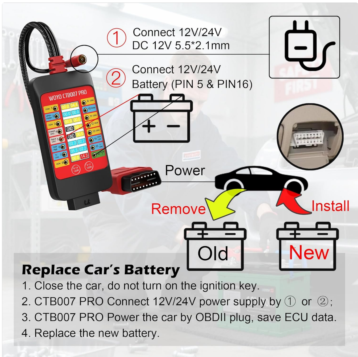
Figure 6: Battery replacement procedure using CTB007 PRO.
