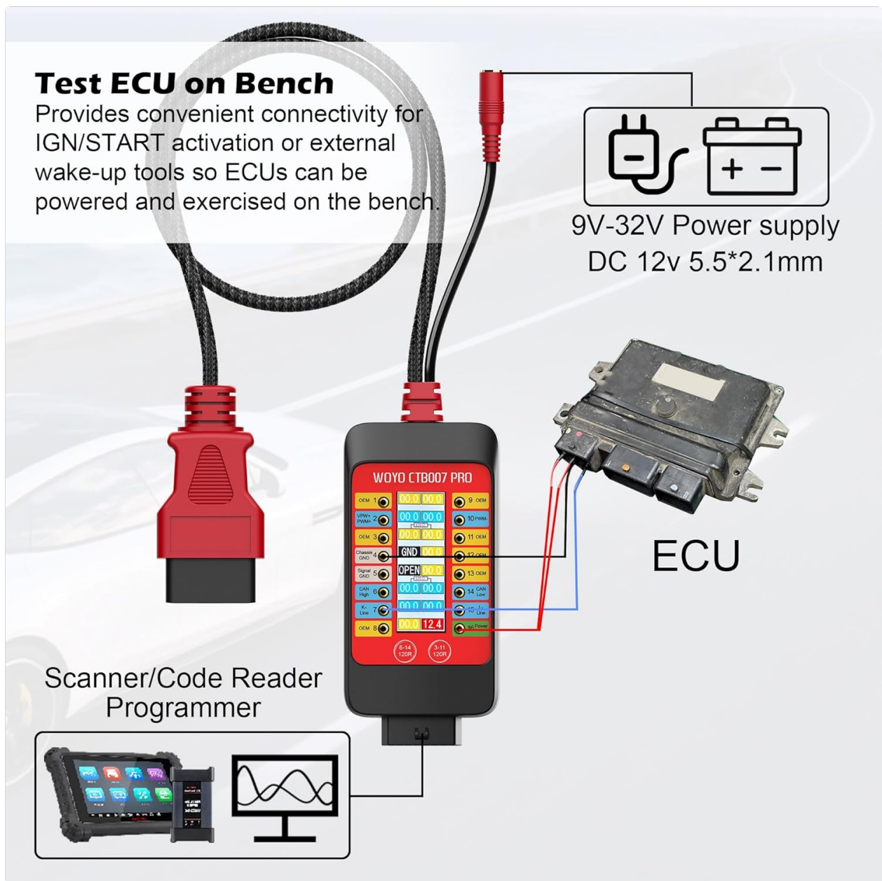
Figure 5: Bench testing an ECU with the CTB007 PRO.
