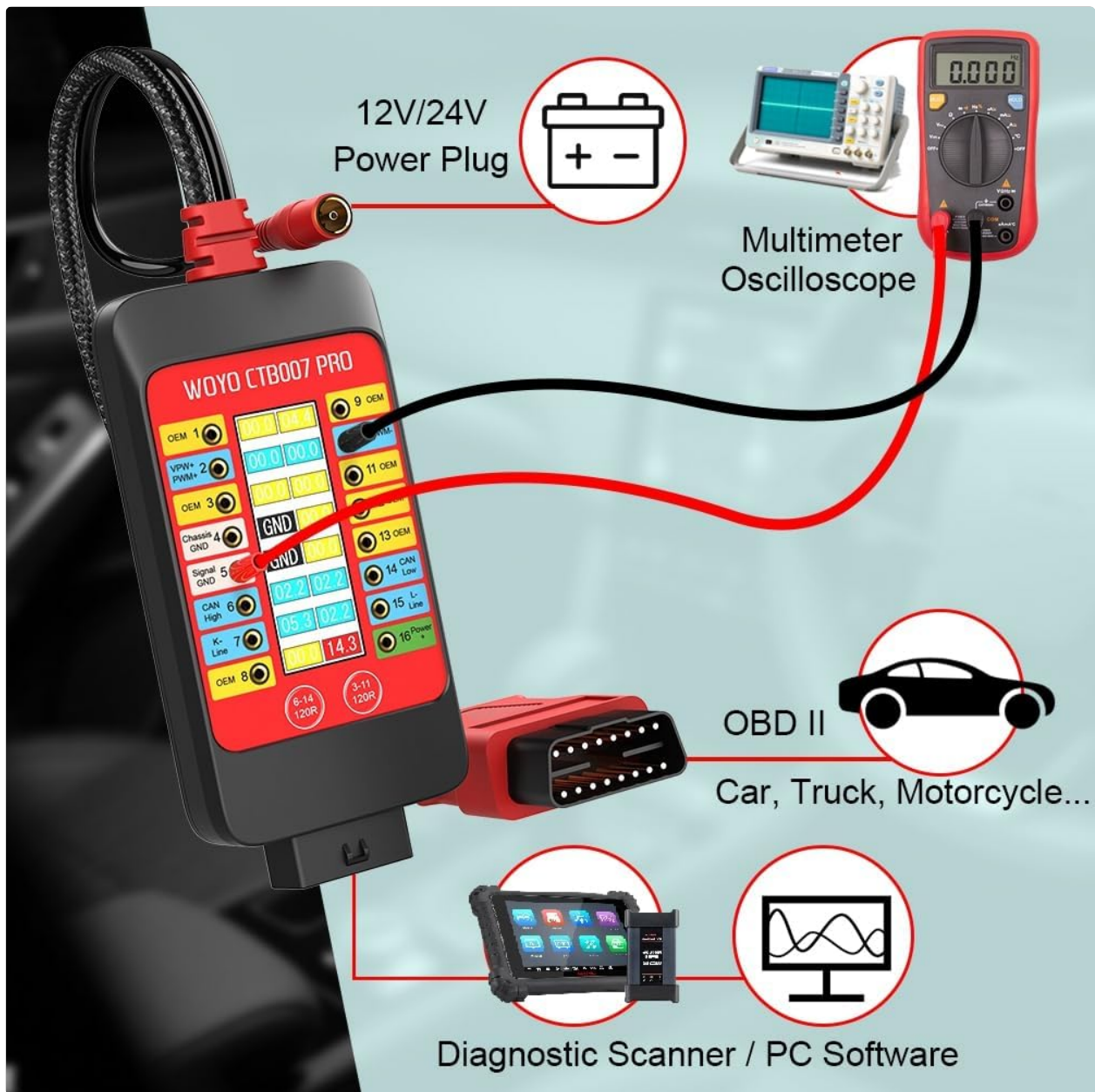
Figure 2: Typical setup for vehicle diagnostics using the CTB007 PRO.
