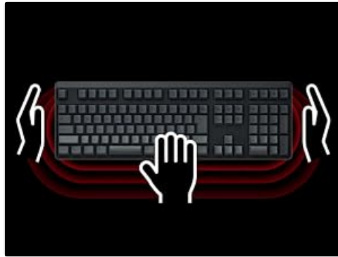
Figure 4.3: The proximity sensor detects user presence for power management.
