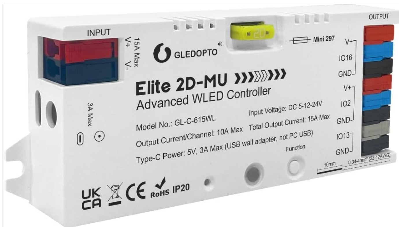
Image 1.1: Front view of the Sogledwow Elite Series ESP32 WLED LED Strip Controller.
