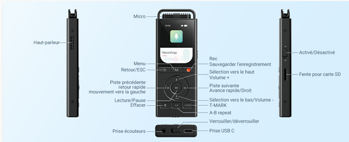
Image: Labeled diagram of the MECHEN V06 recorder.
