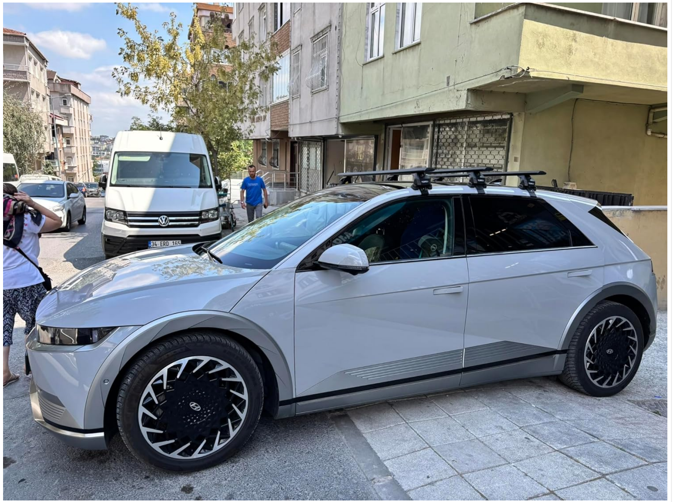
Figure 5: Correct positioning of the cross bars on the vehicle roof.
