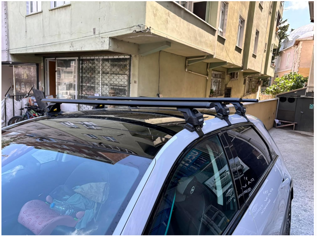
Figure 6: Securing the mounting brackets to the vehicle.
