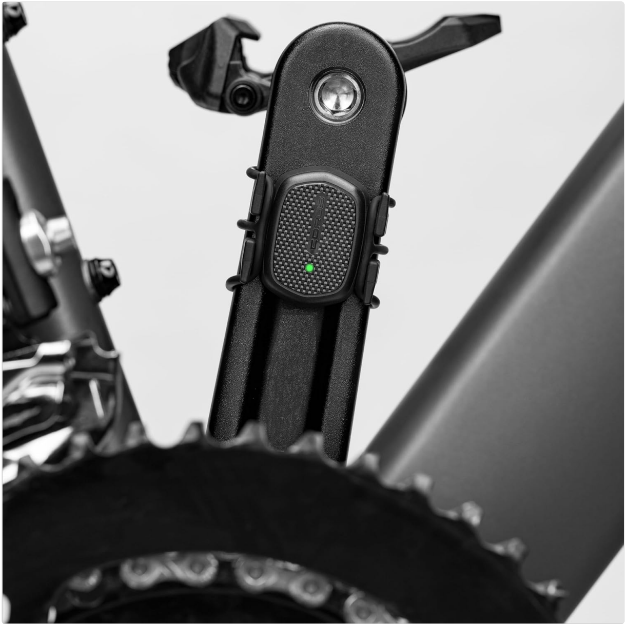
Image: The cadence sensor attached to a bicycle crank arm, ready for use.
