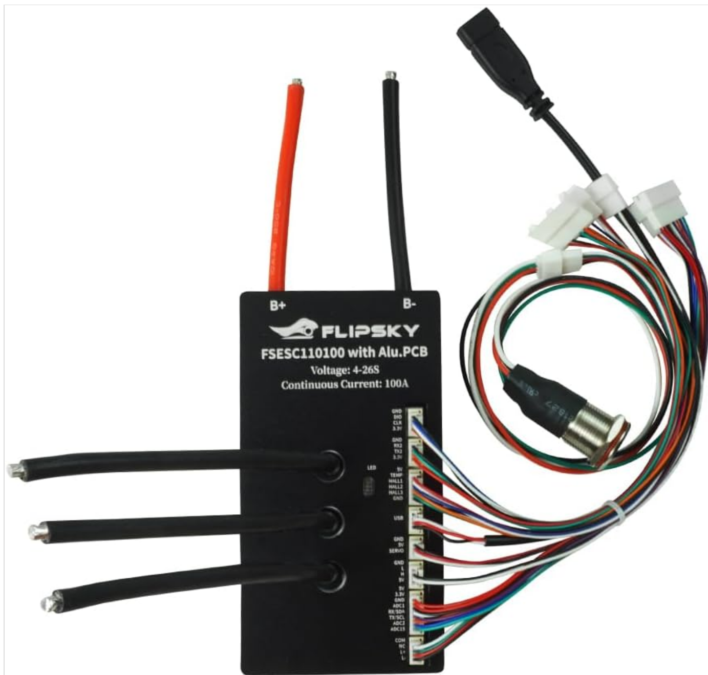
Figure 2.2: The FSESC 110100 ESC along with its various connection cables and accessories, including a USB cable and sensor wires.
