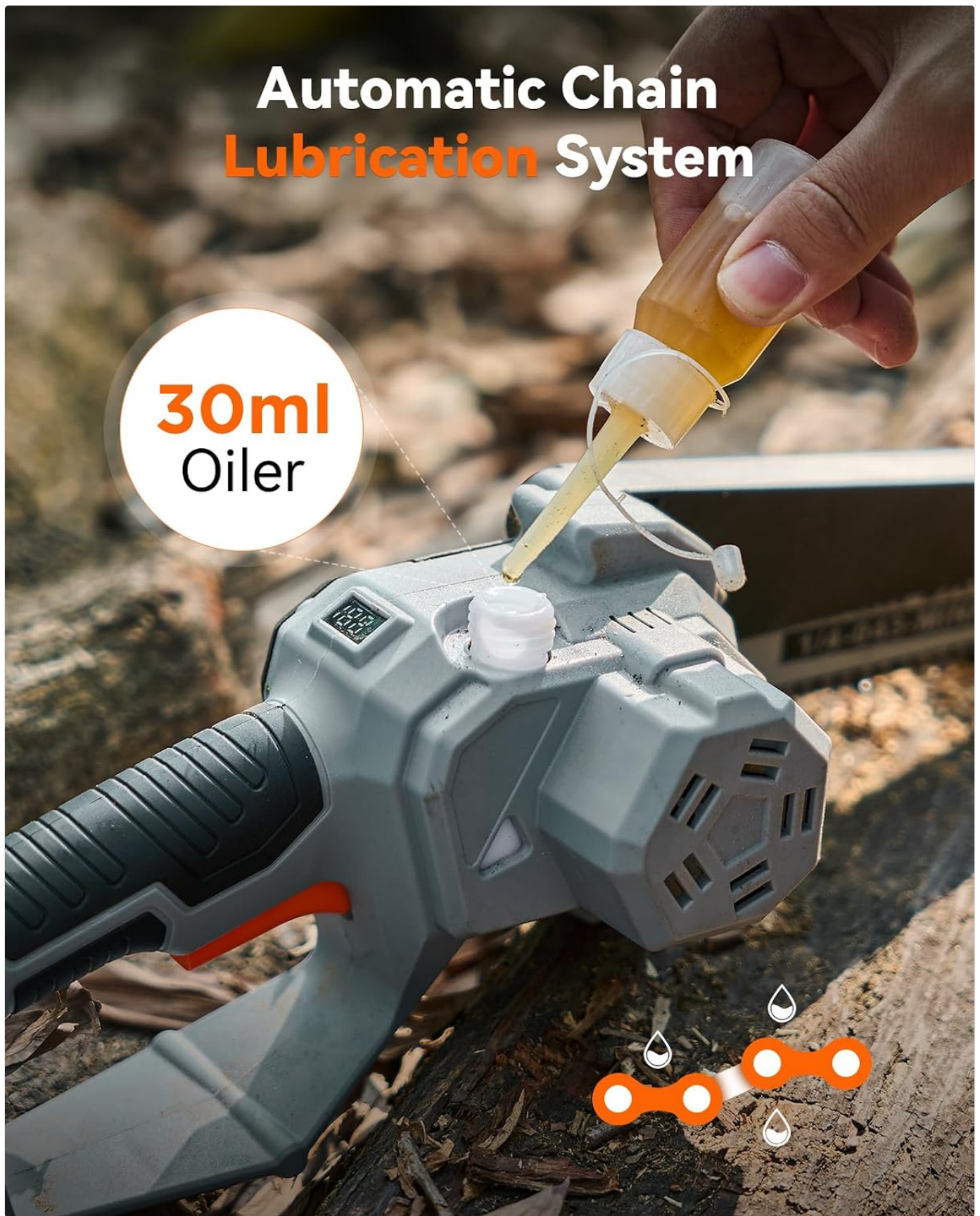
Figure 4.1: Filling the automatic chain lubrication system with chain oil.
