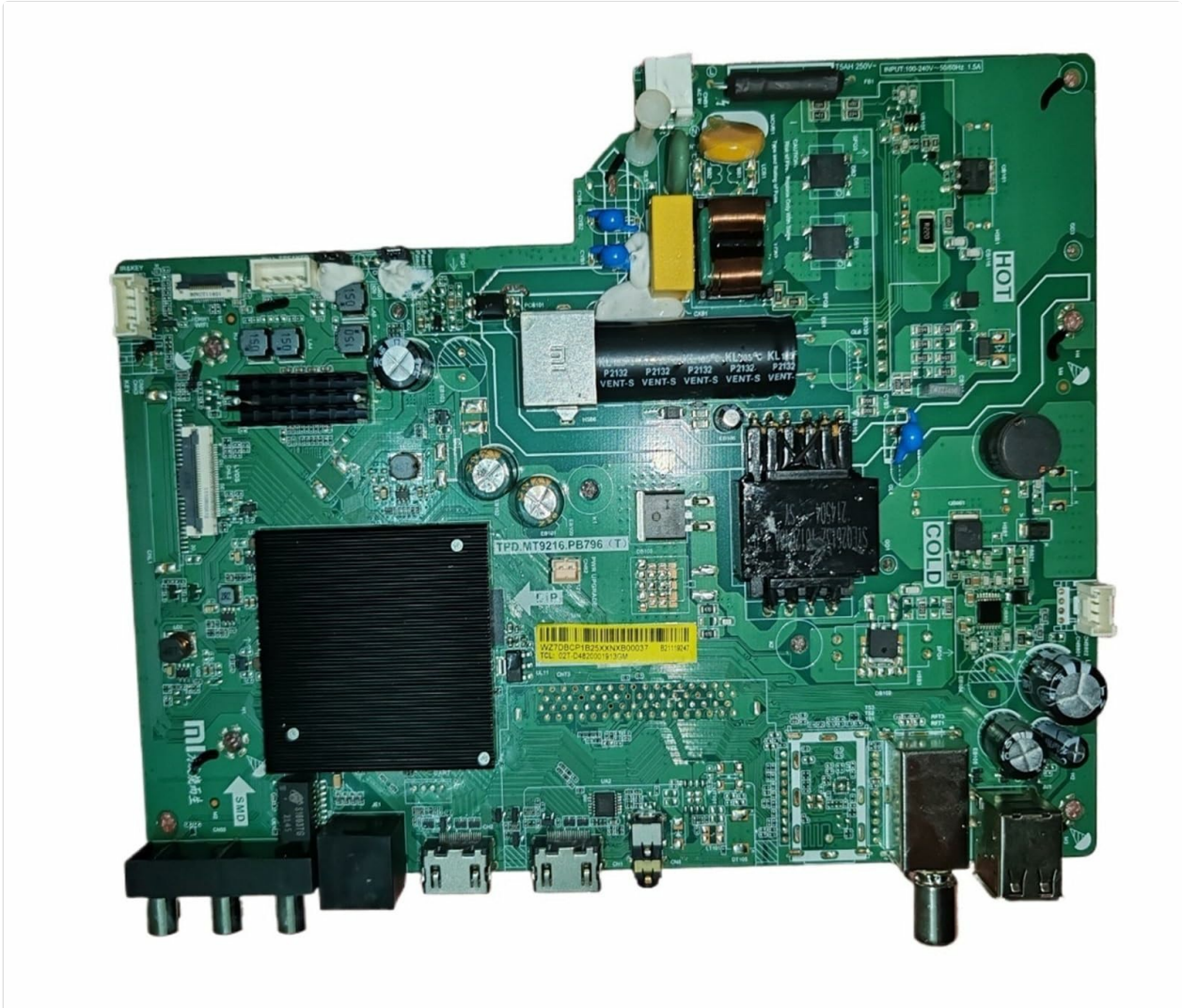
Figure 1: Front view of the TPD.MT9216.PB796(T) B22010379 02T-D182001942GM TV mainboard. This image displays the primary processing unit (under the heatsink), memory modules, power regulation components, and various input/output ports including HDMI, USB, and antenna connectors.
