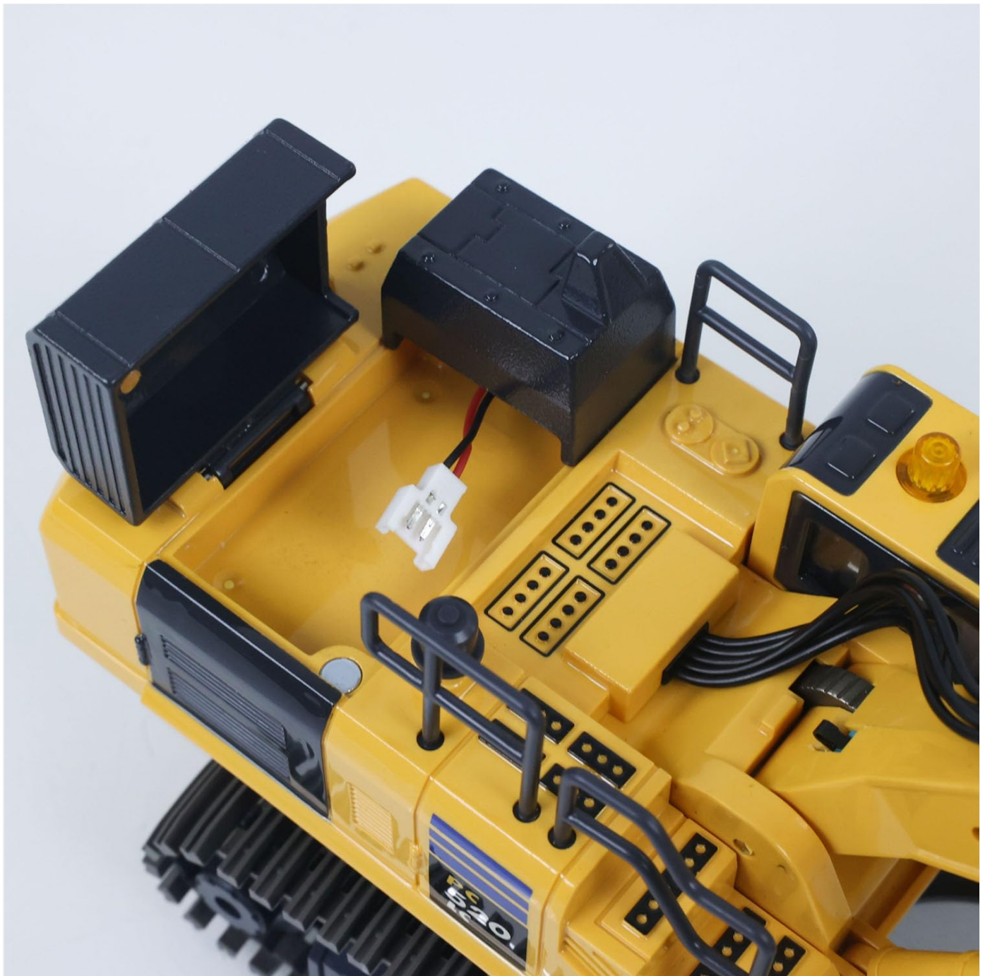
Image: Close-up view of the excavator's battery compartment, showing the connector for the rechargeable battery.
