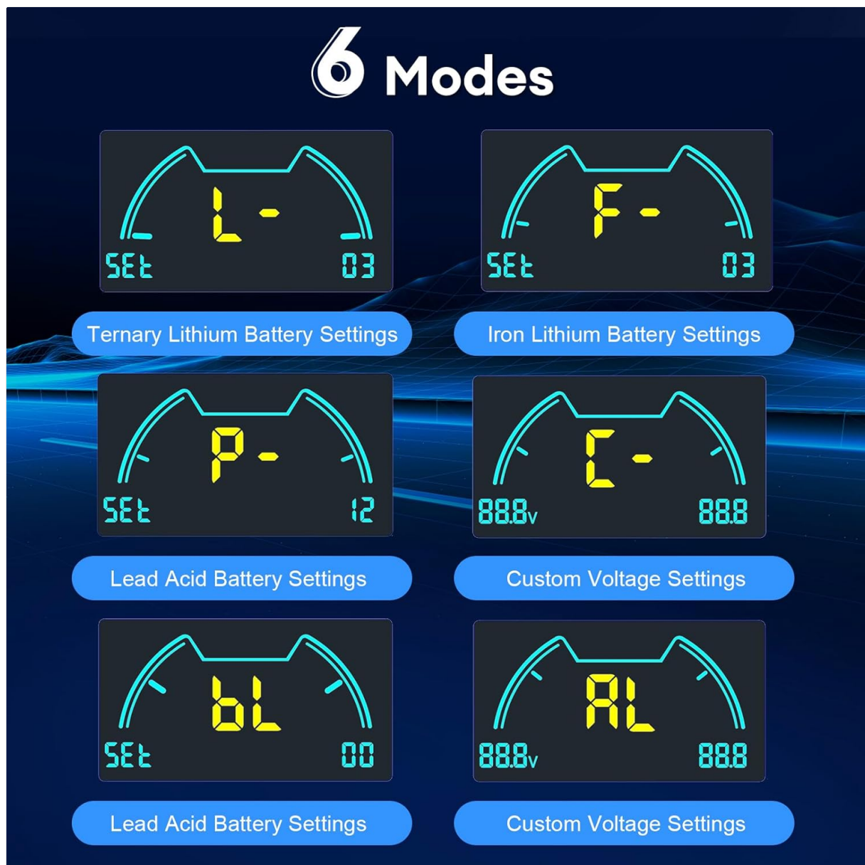
Figure 4: Overview of the six configurable modes for the diymore battery meter.
