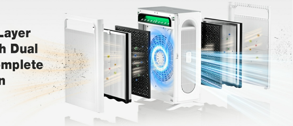
Image 4.1: Detailed view of the dual 3-stage filtration system, illustrating the washable pre-filter, True HEPA filter, and activated carbon filter.
