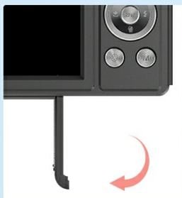
Step 1: Open battery cover.
