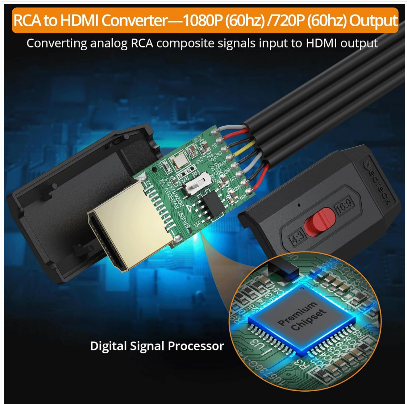
Image: Internal view of the Neoteck RCA to HDMI converter, highlighting the digital signal processor and integrated cables.
