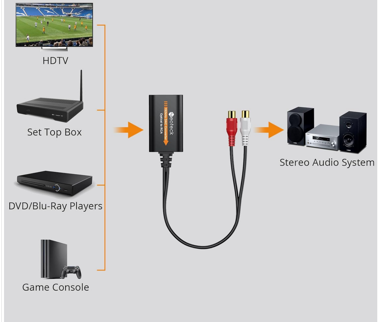
Image: Diagram showing how to connect the Optical to RCA DAC converter from an HDTV, set-top box, DVD/Blu-ray player, or game console to a stereo audio system.
