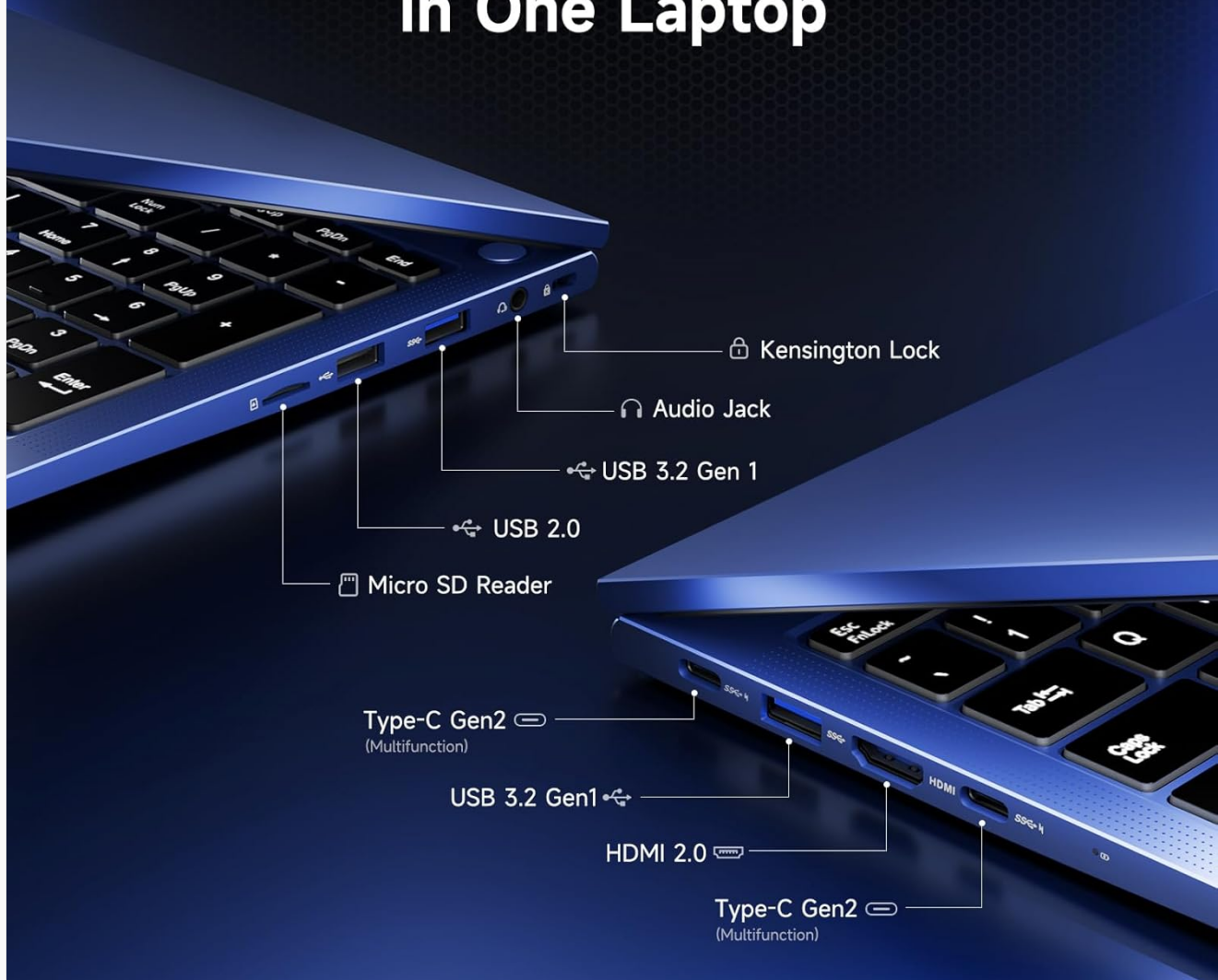
Figure 3.4: Detailed view of the laptop's ports and their functions.
