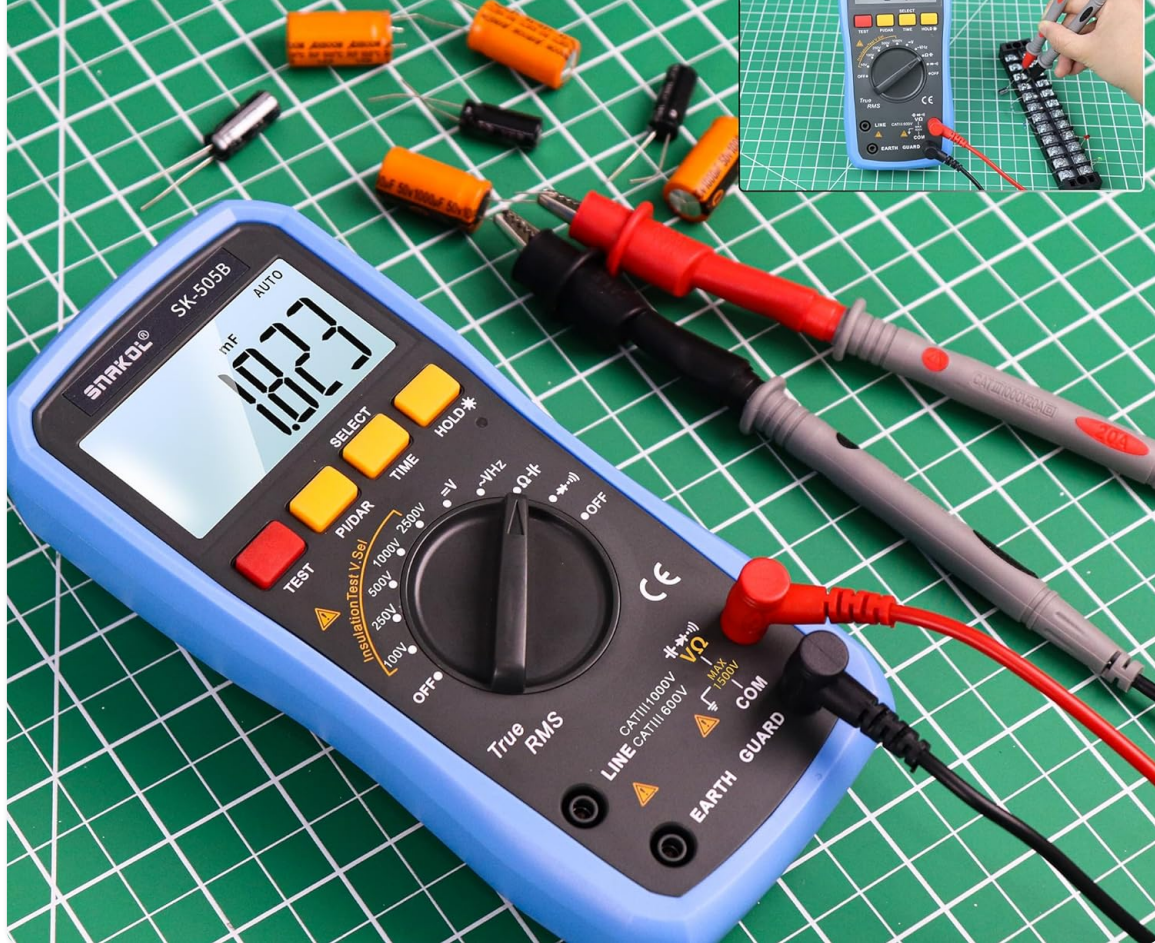
Figure 6: The SK-505A measuring capacitance, demonstrating its ability to measure up to 100mF.
