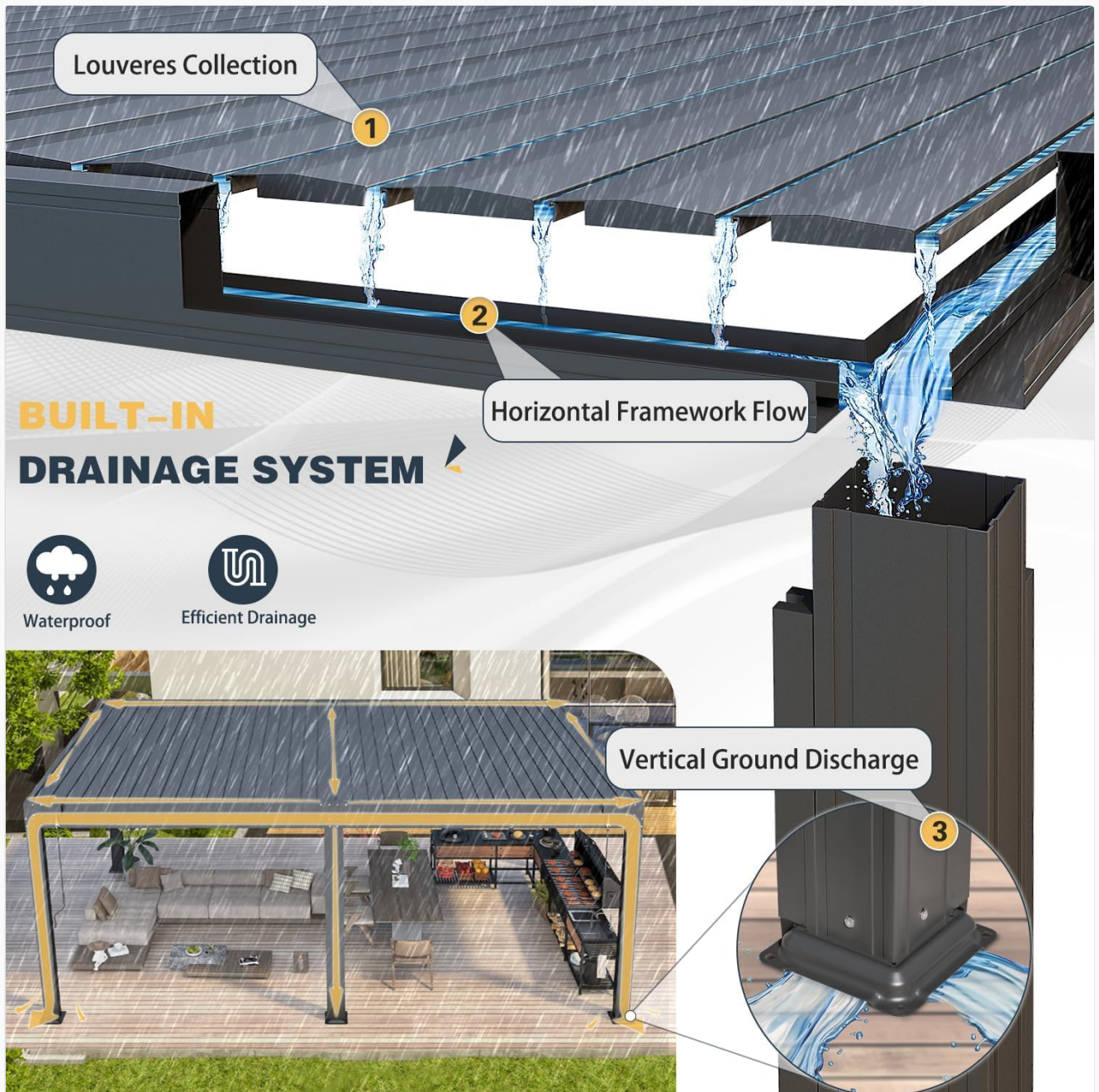
Image: A detailed diagram illustrating the pergola's built-in drainage system, showing rainwater collection by louvers, horizontal flow through the framework, and vertical discharge through the legs.
