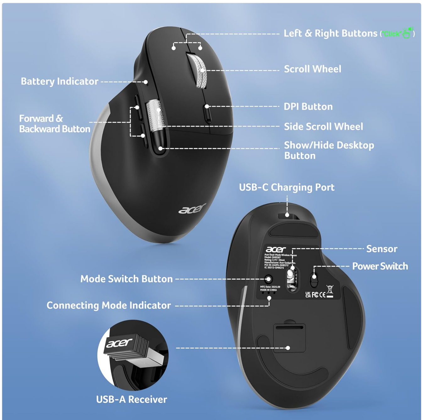
Figure 3: Acer Ergonomic Wireless Mouse - Labeled Components.
