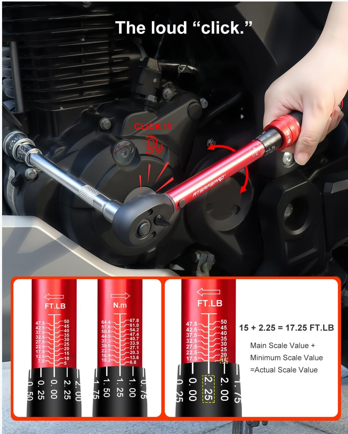
Image: Illustration of the audible "click" mechanism and a detailed view of the dual scale for precise torque reading.
