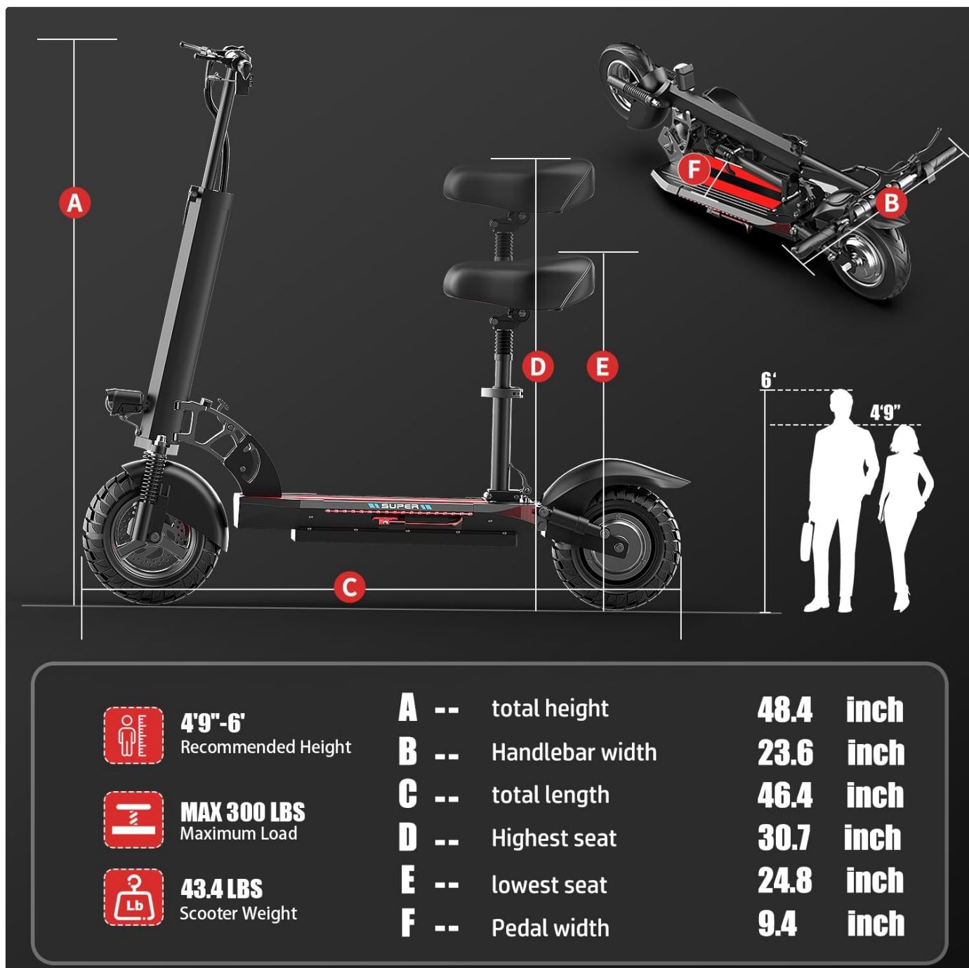
Image 8.2: Dimensional specifications of the ASKGO Q2 Electric Scooter.
