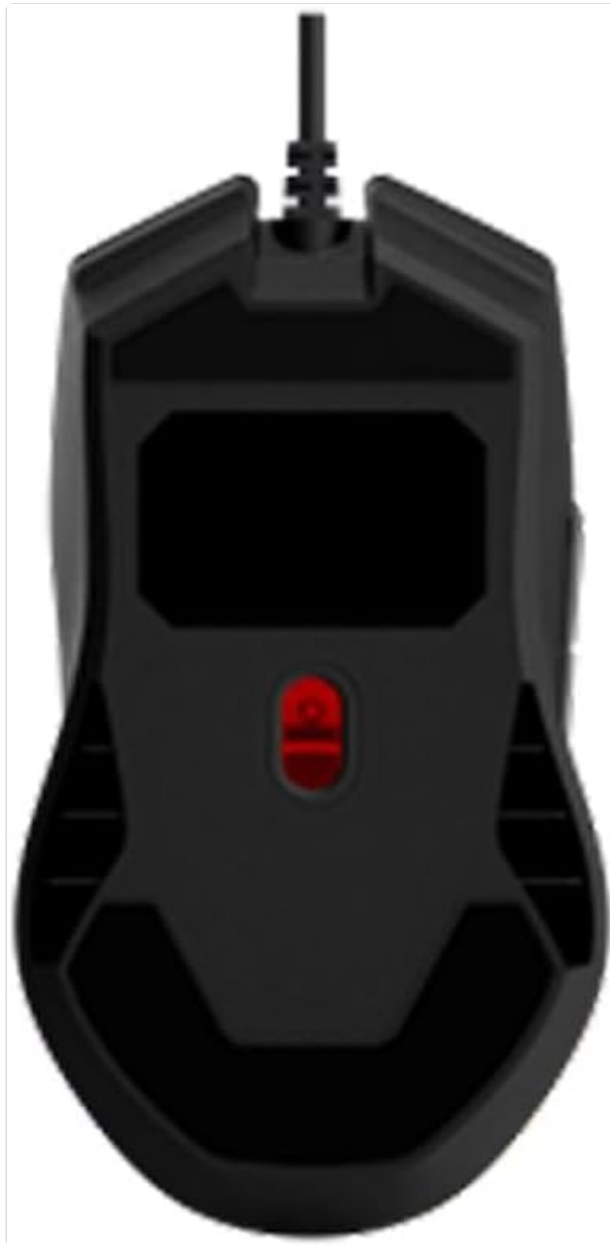
Figure 4: Underside of the mouse, indicating the location of the optical sensor.
