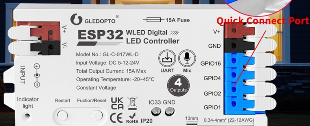
Image 1.1: Overview of the GL-C-017WL-D controller highlighting its key features: 15A fuse, audio-reactive microphone, segmental control, and Type-C UART download port.
