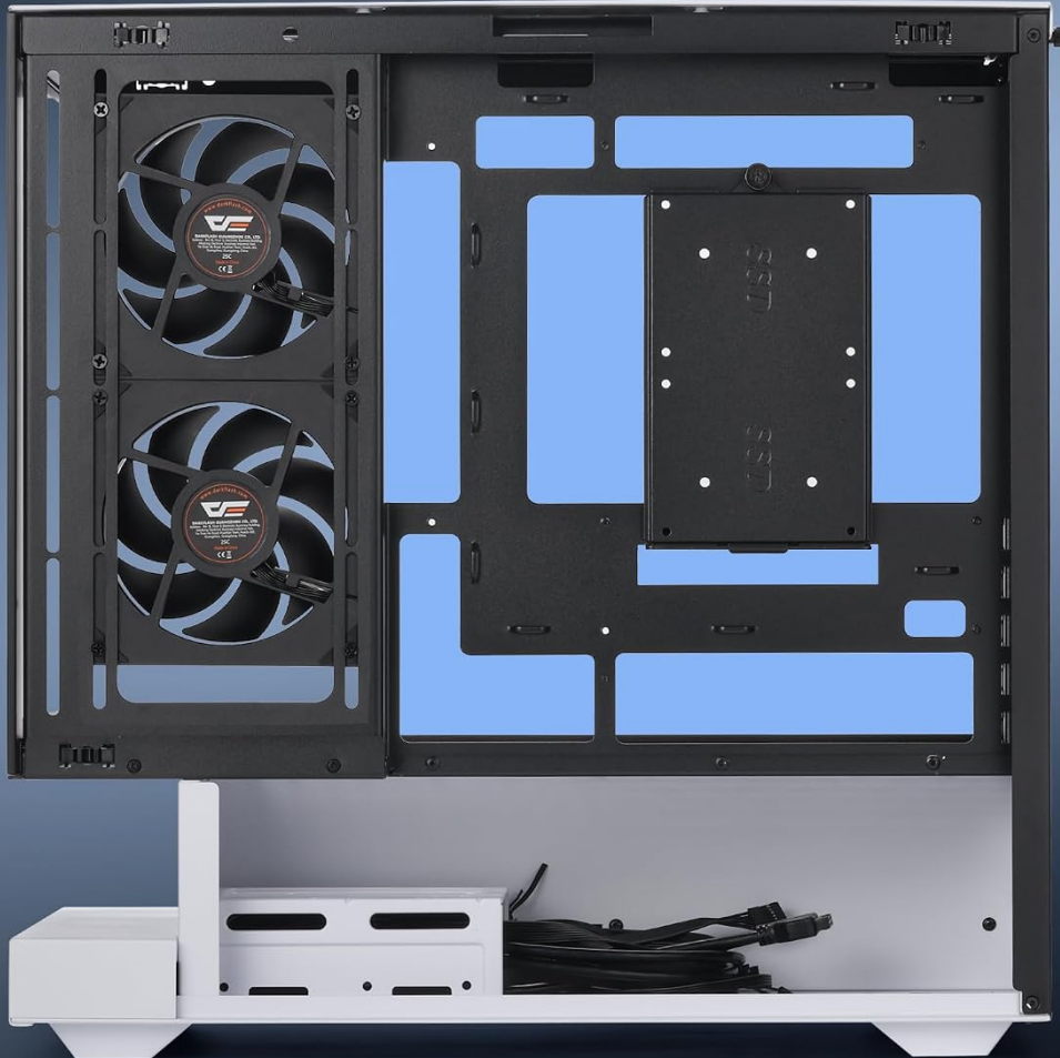
Image 4.2: Internal view of the darkFlash FLOATRON F1 highlighting the design for back-connect motherboard support, which aids in cable management.
