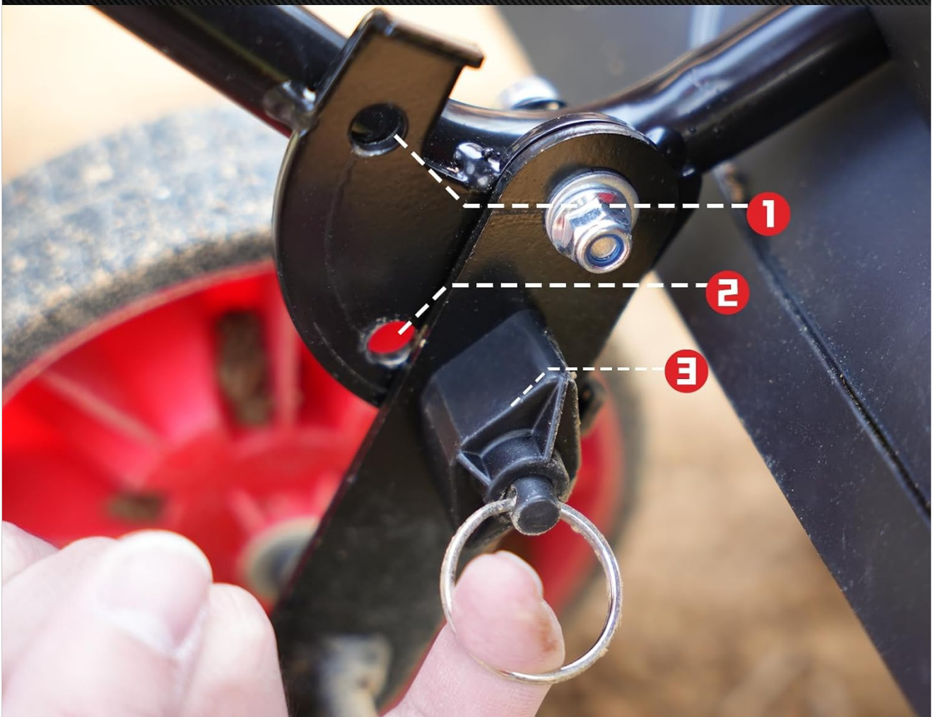
Figure 1: Adjusting the 3-position wheels for desired tilling depth.
