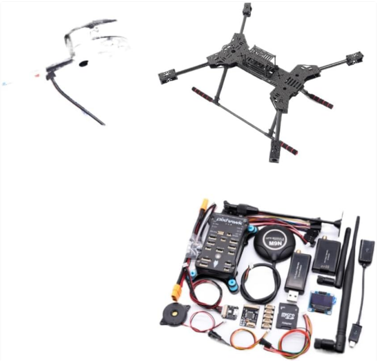
Image 1: Overview of the ZD680 Hexacopter Frame Kit and included components.
