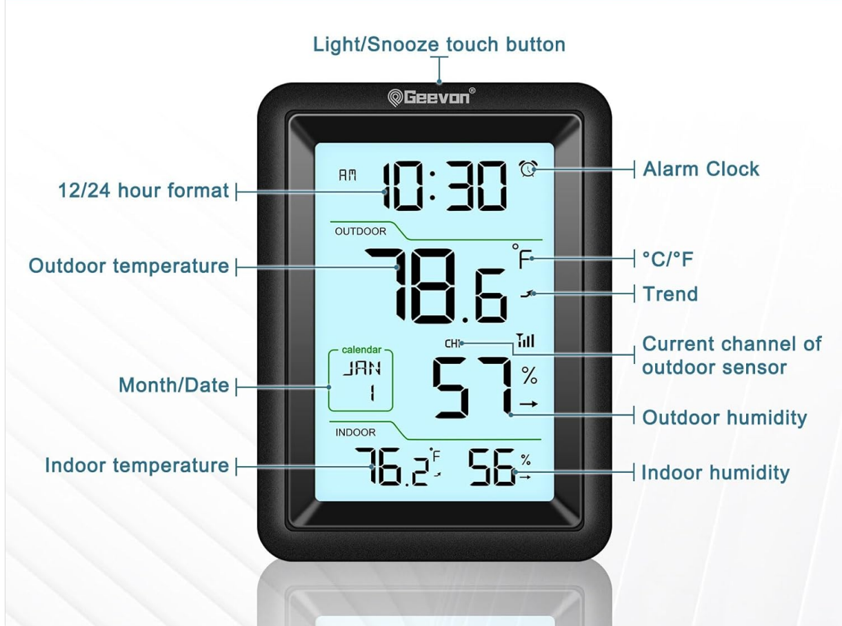
Figure 1: Main unit display with key features labeled, including time, date, indoor/outdoor temperature and humidity, and trend indicators.
