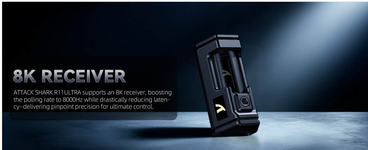
Image 4.1: The 8K wireless receiver, which enables an 8000Hz polling rate for the ATTACK SHARK R11 Ultra mouse.
