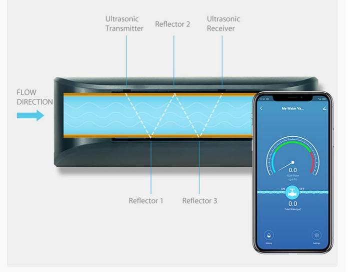
An internal diagram of the Haozee Smart Water Valve, detailing the W-type ultrasonic technology used for accurate water flow detection, showing the transmitter, reflectors, and receiver.
