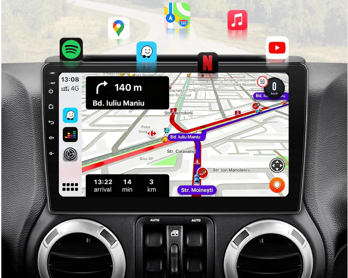
Image 4.2: The car radio display showing GPS navigation in progress, with icons for various apps like Spotify, YouTube, and Google Maps, illustrating WiFi and GPS capabilities.
