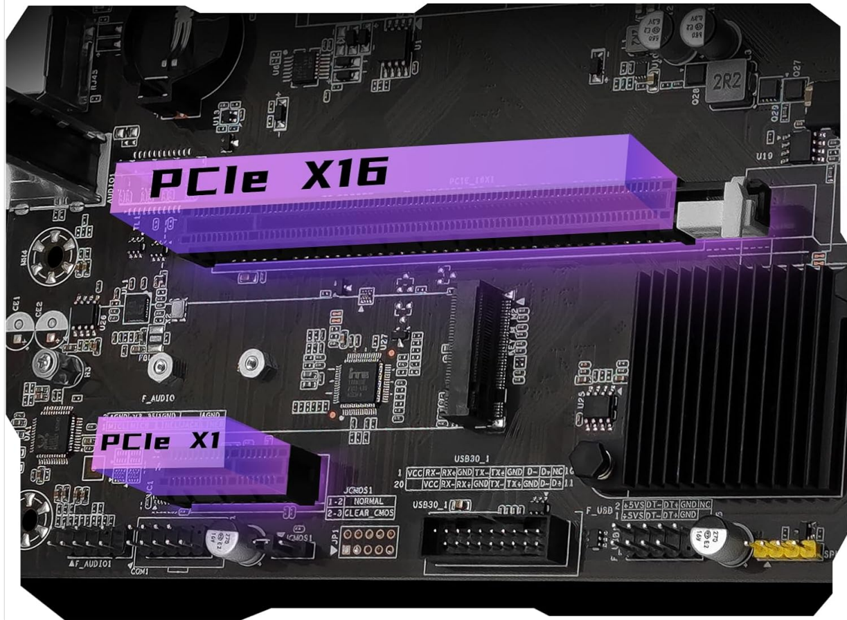
Image 2.5: The PCIe 3.0 x16 and PCIe 2.0 x1 slots on the motherboard, used for graphics cards and other expansion devices.
