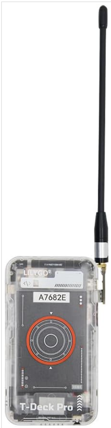
Back view of the LILYGO T-Deck Pro, showing the transparent casing and the A7682E module.
