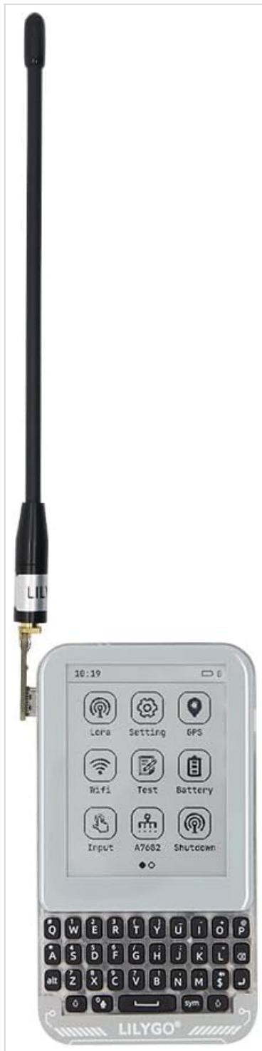
Front view of the LILYGO T-Deck Pro, displaying the e-paper screen and QWERTY keyboard.
