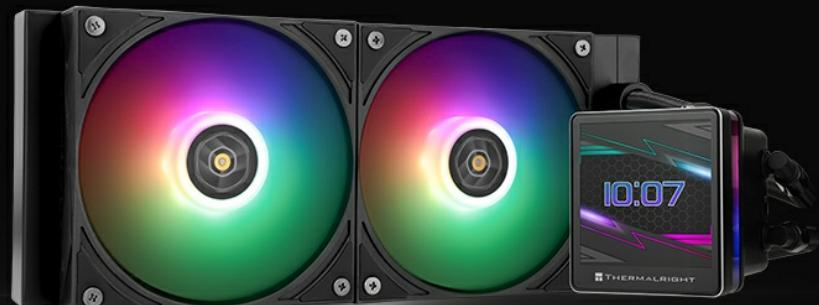
The 3.4-inch IPS LCD screen provides real-time monitoring of system metrics like CPU and GPU temperatures, along with customizable visuals.
