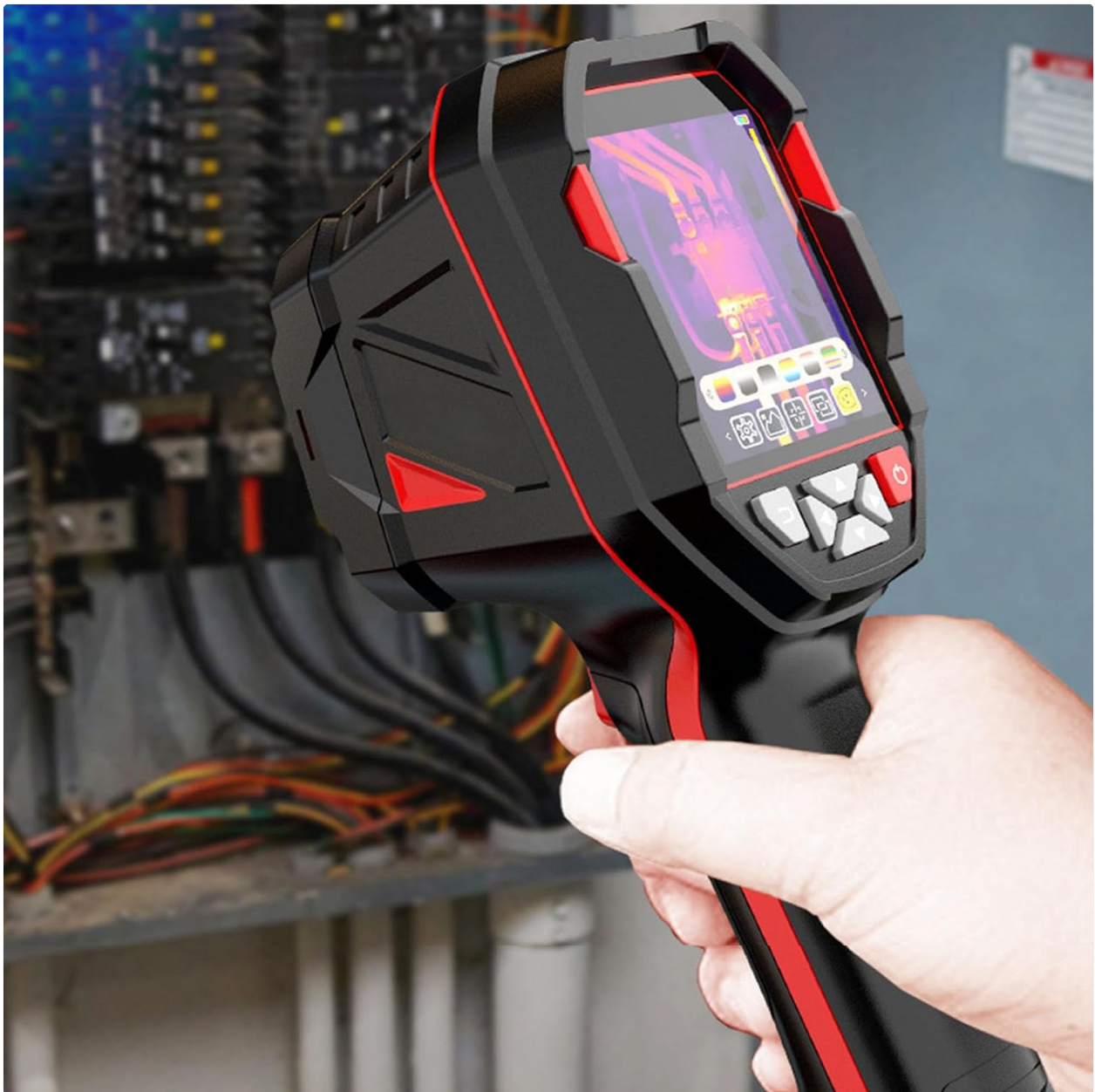
Figure 4.1: The HT821A in use, demonstrating its application in inspecting electrical panels for thermal anomalies.
