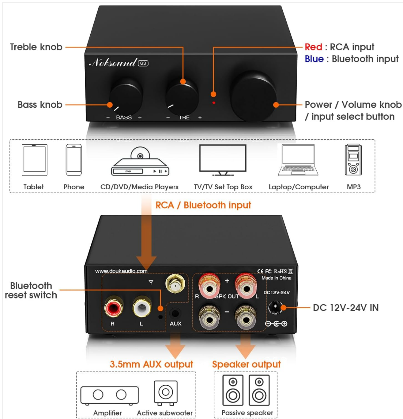
Image 3: Diagram illustrating the front panel controls (Bass, Treble, Power/Volume/Mode knob) and rear panel connections (RCA input, Bluetooth antenna port, 3.5mm AUX pre-out, speaker outputs, DC power input).
